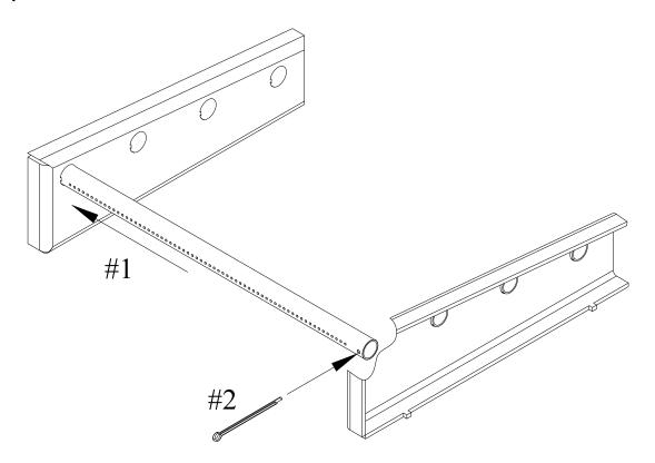
Figure 4.11 – Secondary air tube replacement
